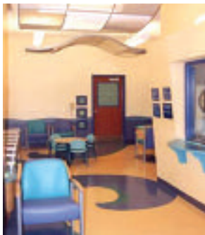
Rapidly renewable materials (credit MR 6) can be used in interiors by incorporating wheatboard into casework and installing linoleum flooring. Shown is the Pediatrics center at St. Luke Hospital in Florence, Kentucky.
